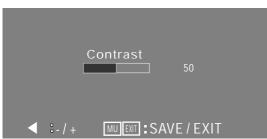
Press button 2: adjust contrast to brighten level. Press button 3: adjust contrast to darken level. Press button 1 to confirm setting. [Contrast adjustable level: 0-100. Preset: 50]
